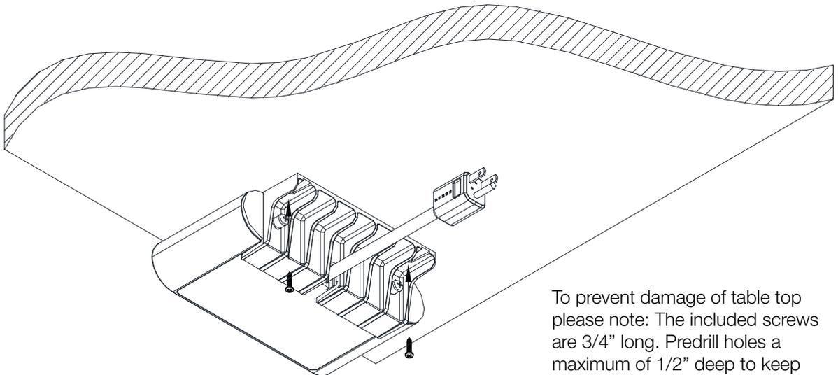
To prevent damage of table top please note: The included screws are 3/4" long. Predrill holes a maximum of 1/2" deep to keep from drilling through the table top. Over tightening of screws during installation or adjustments can damage the product and affect the function and warranty.
