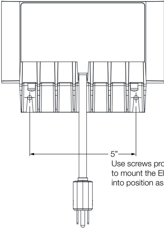
Use screws provided to mount the Ellipse into position as shown.
