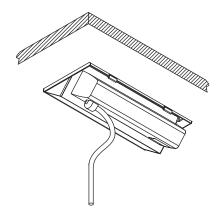
Note: In a conduit application, conduit should be supported according to local code. When managing conduit and cabling exiting the unit, ensure there is adequete slack to allow unit to open properly
