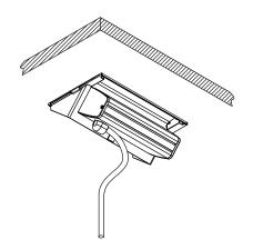
Note: In a conduit application, conduit should be supported according to local code. When managing conduit and cabling exiting the unit, ensure there is adequate slack to allow unit to open properly
