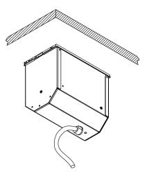
Note: In a conduit application, conduit should be supported according to local code. When managing conduit and cabling exiting the unit, ensure there is adequete slack to allow unit to open properly
