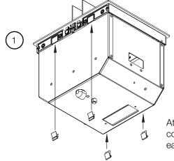
Attach 2 clips at the connect points along each side of the unit.
