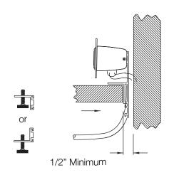
Tighten the knob until the unit is secure.
